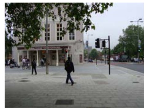
The pedestrian streetscape continues at crossings indicating priority over traffic.
